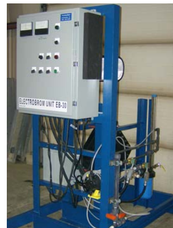
Electrolytic Bromine Unit
